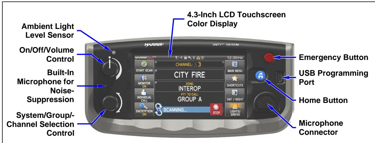
Figure 8-3: CH-100 Control Head Front Panel
