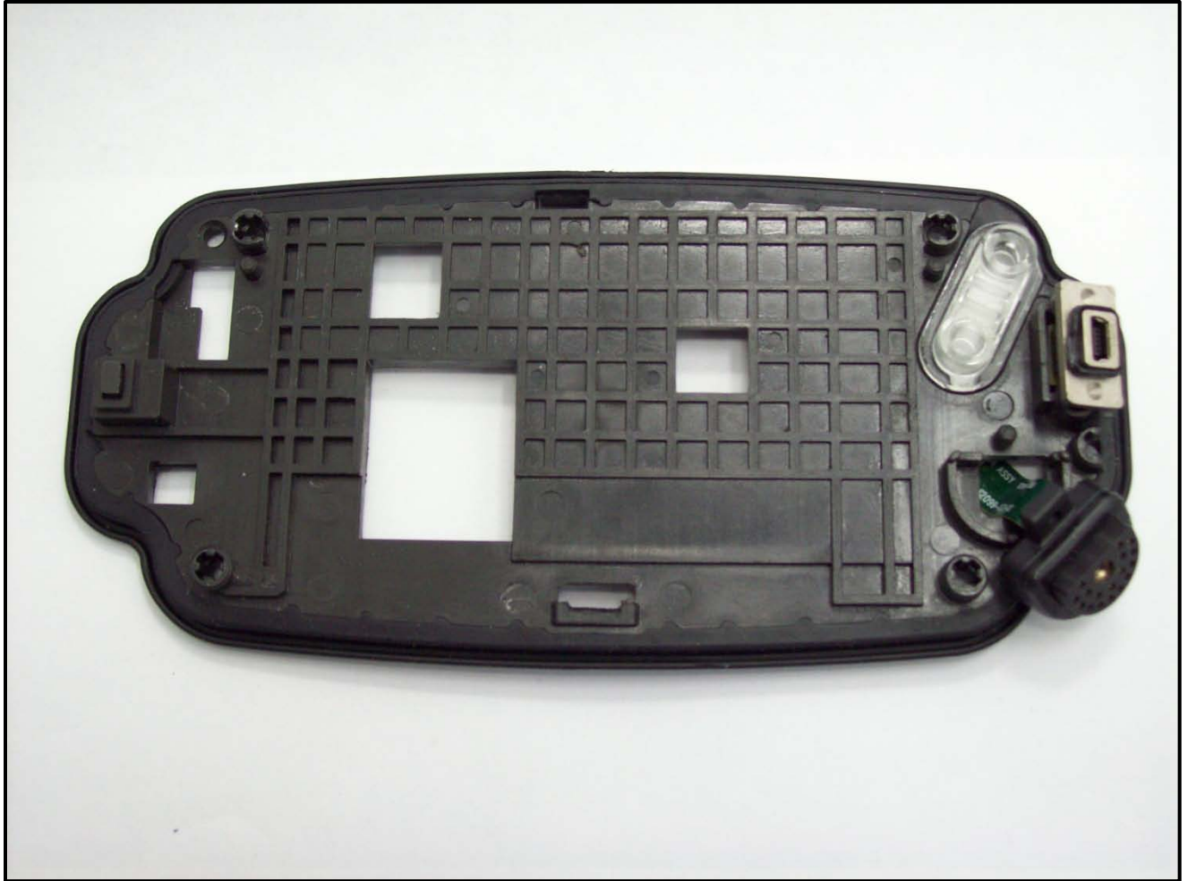
Photograph 24: Control Head Gasket
