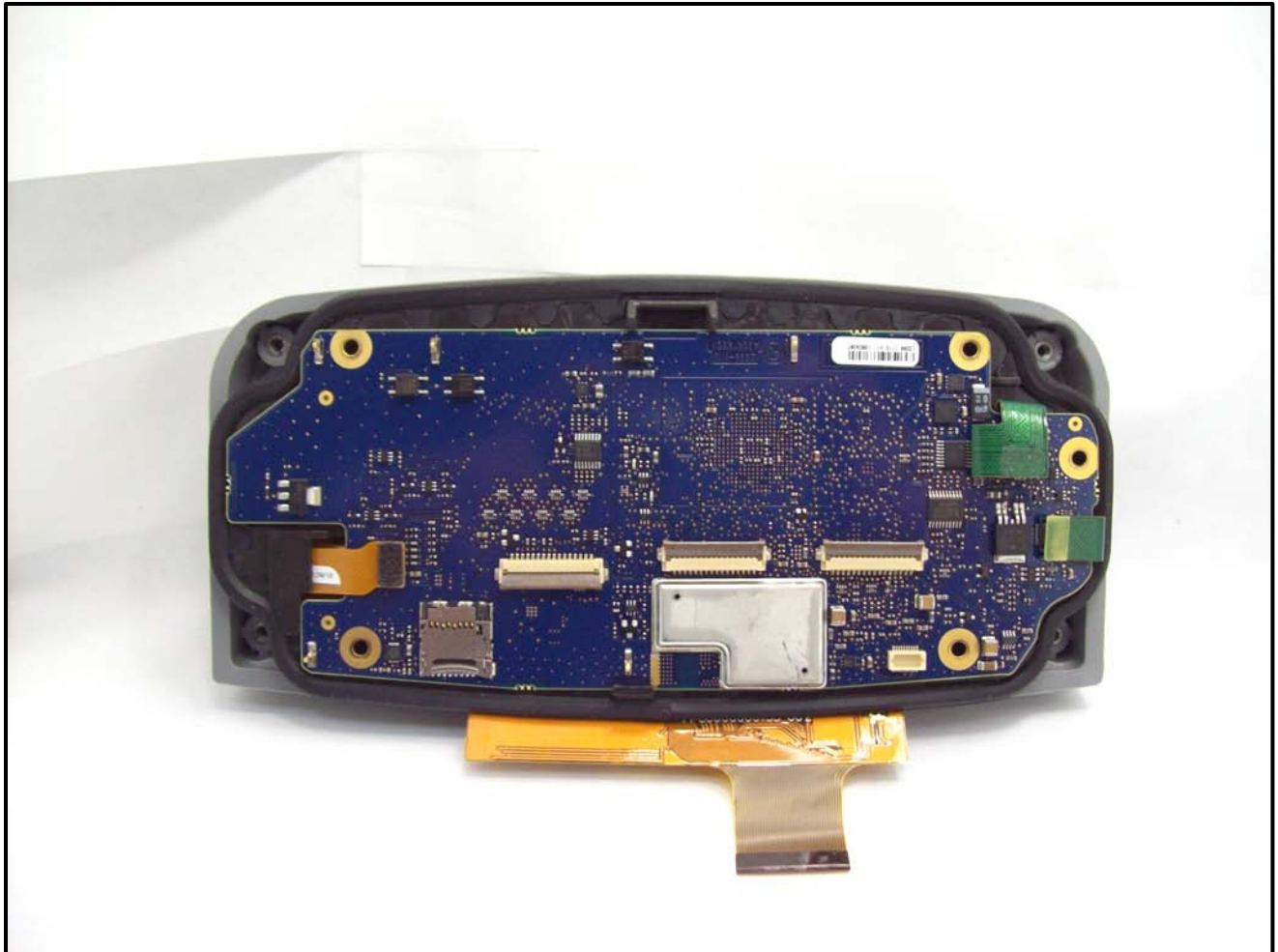
Photograph 22: Back Half of Control Head 1
