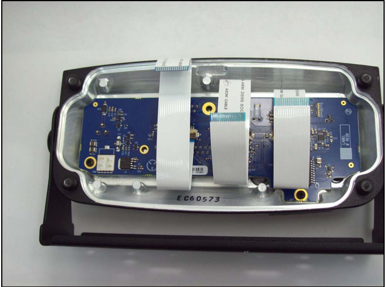
Photograph 23: Back Half of Control Head 2
