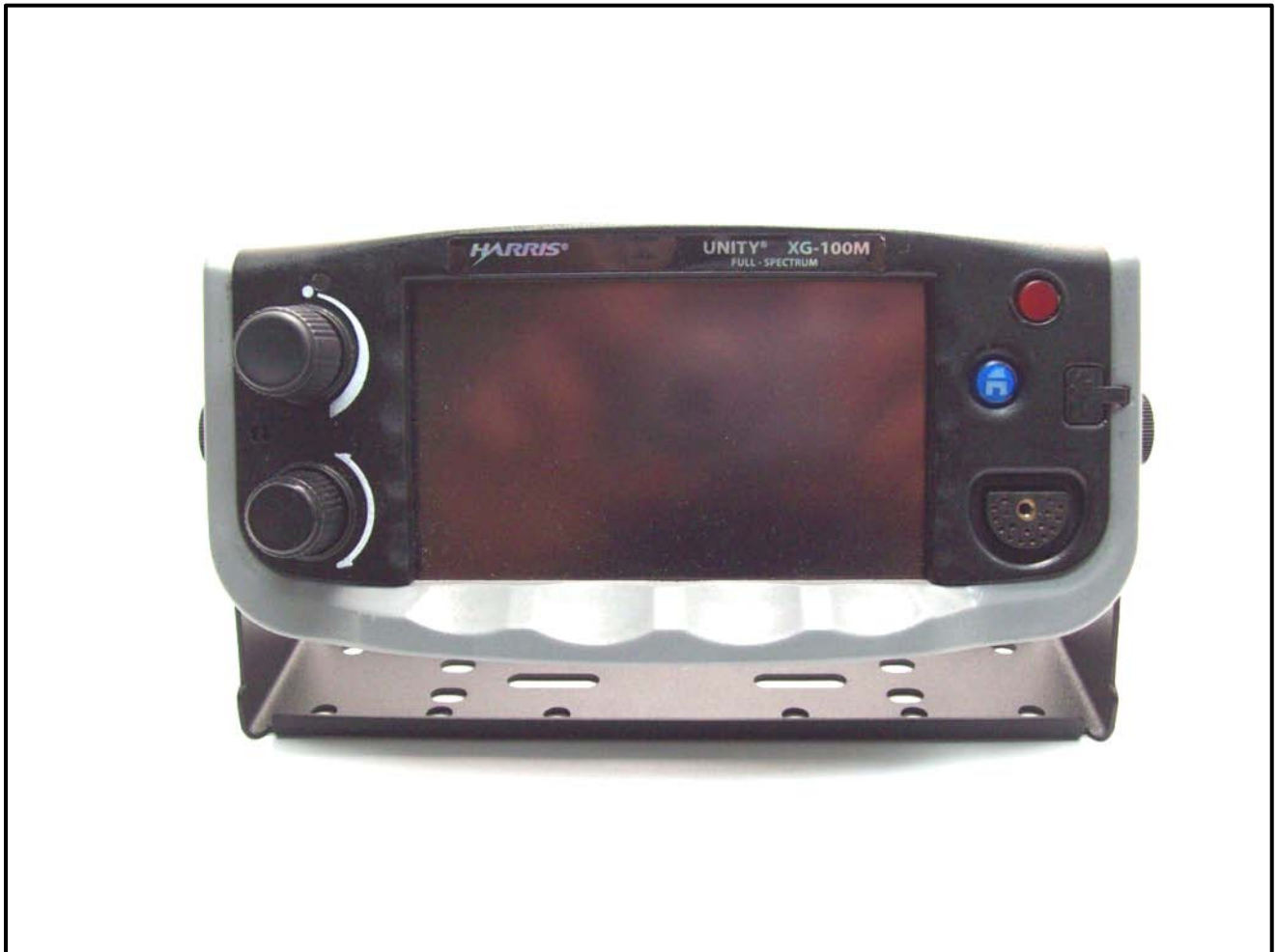
Photograph 6: Control Head for Remote Operation - Front
