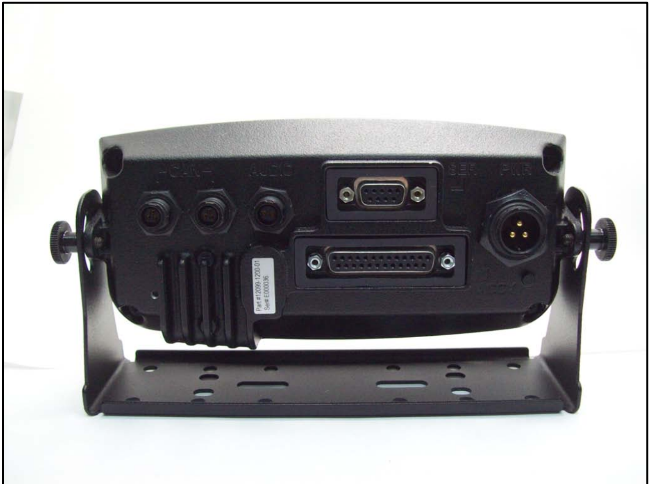
Photograph 7: Control Head for Remote Operation – Back
