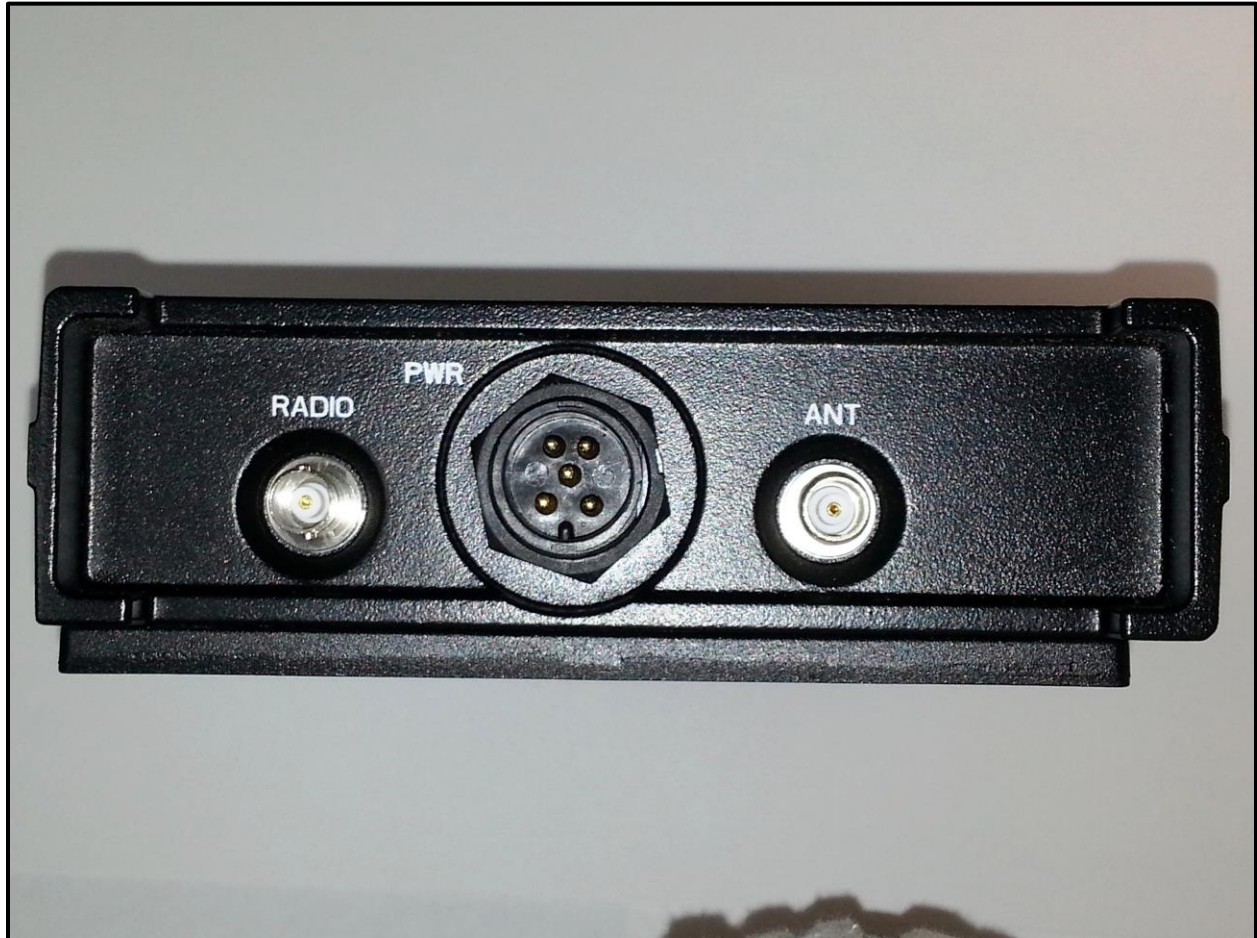
Photograph 6: Back View – Connectors
