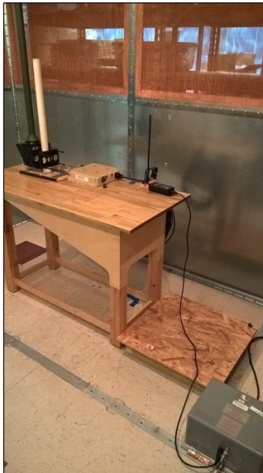
Photograph 18. Conducted Emissions, Omni 8, Test Setup
