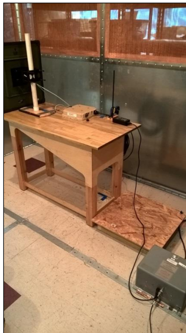
Photograph 14. Conducted Emissions, 2' Panel, Test Setup
