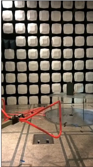
Photograph 11. Undesirable Emissions, 90 Sector Below 1 GHz
