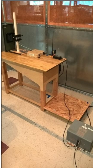
Photograph 17. Conducted Emissions, 90 Sector. Test Setup
