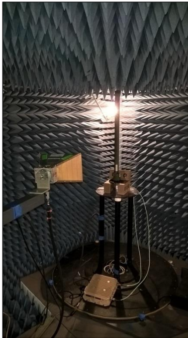
Photograph 10. Undesirable Emissions, 8 Omni Above 1 GHz
