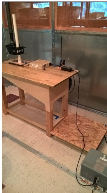
Photograph 16. Conducted Emissions, 5 Omni, Test Setup
