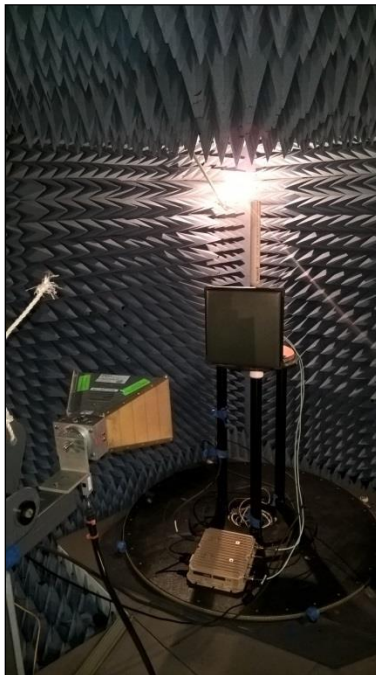
Photograph 2. Undesirable Emissions, 1' Panel Above 1 GHz
