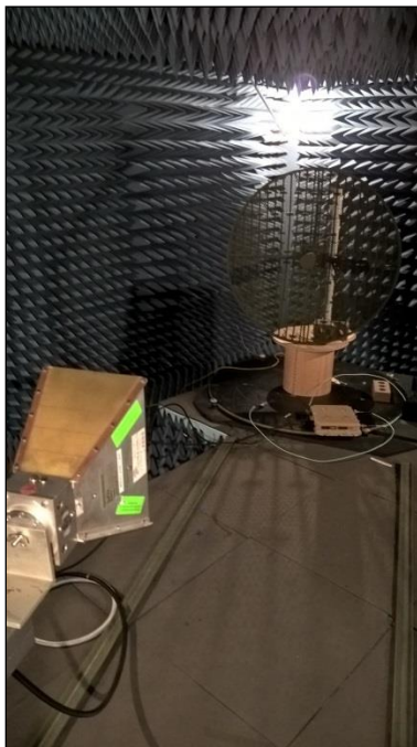
Photograph 6. Undesirable Emissions, 3' Para Above 1 GHz
