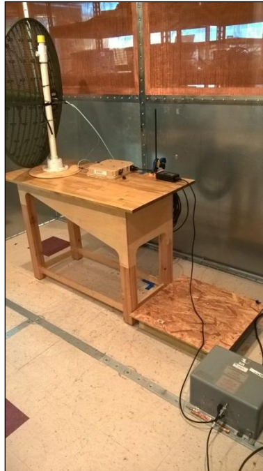
Photograph 15. Conducted Emissions, 3' Para, Test Setup
