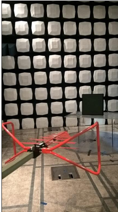
Photograph 3. Undesirable Emissions, 2' Panel Below 1 GHz
