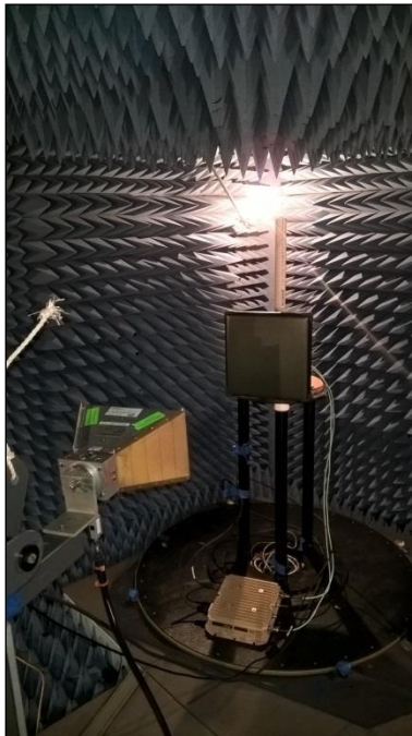
Photograph 2. Undesirable Emissions, 1' Panel above 1 GHz, Test Setup
