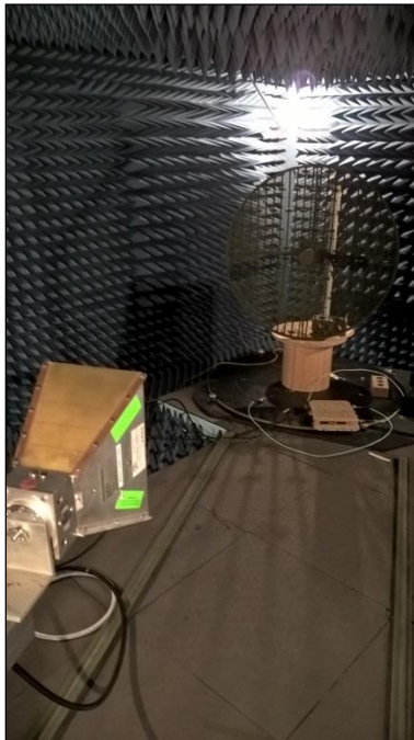
Photograph 6. Undesirable Emissions, Para above 1 GHz, Test Setup
