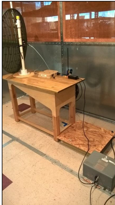
Photograph 15. Conducted Emissions, 3' Para, Test Setup
