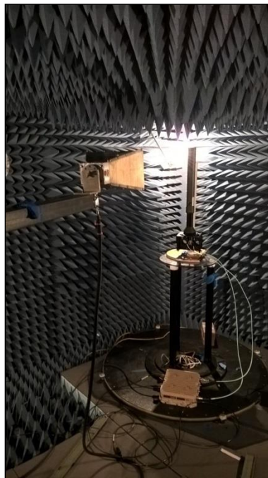
Photograph 8. Undesirable Emissions, 5 Omni above 1 GHz, Test Setup
