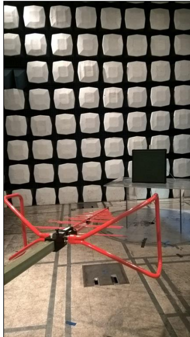
Photograph 3. Undesirable Emissions, 2' Panel below 1 GHz, Test Setup
