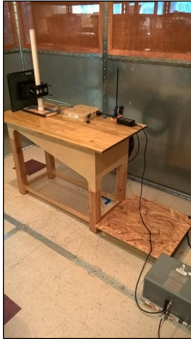
Photograph 13. Conducted Emissions, 1' Panel, Test Setup
