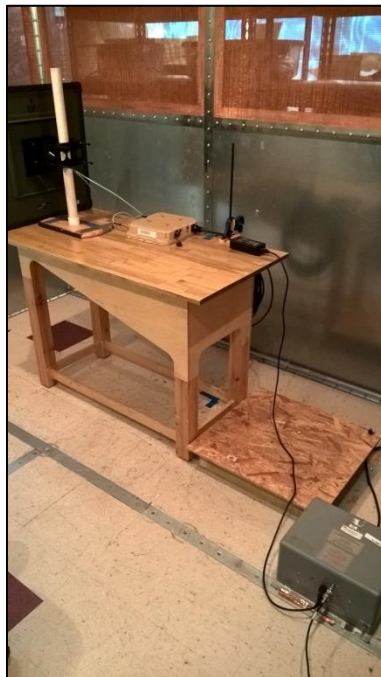
Photograph 14. Conducted Emissions, 2' Panel, Test Setup
