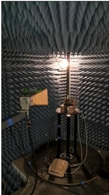
Photograph 10. Undesirable Emissions, 8 Omni above 1 GHz, Test Setup
