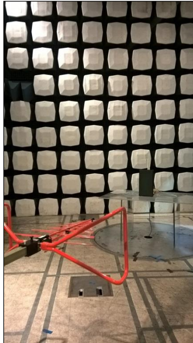
Photograph 11. Undesirable Emissions, 90 Sector below 1 GHz, Test Setup
