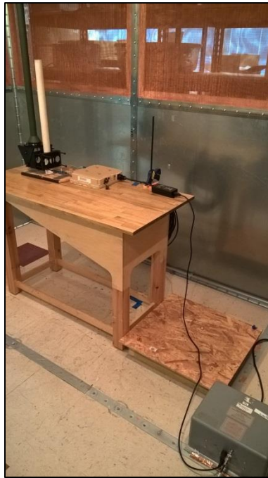
Photograph 17. Conducted Emissions, Omni 8, Test Setup
