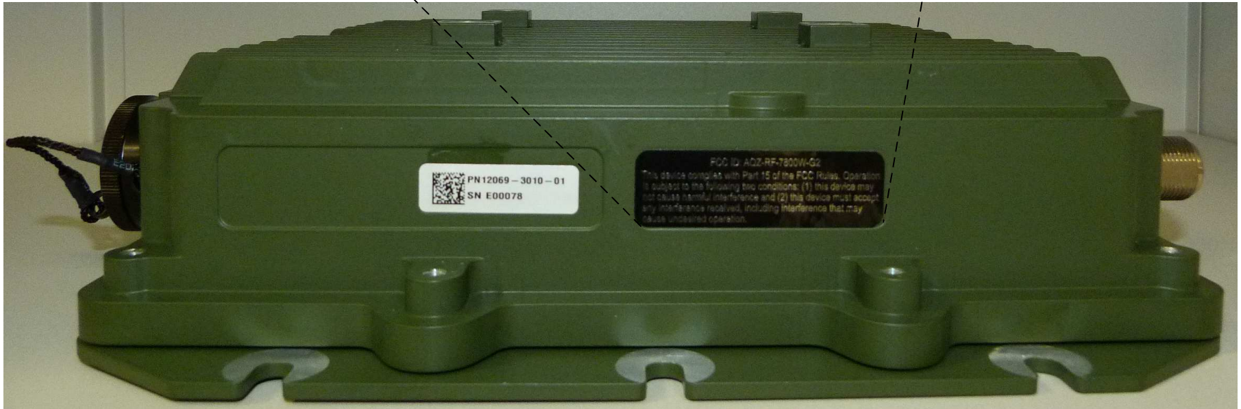
Harris Corporation Broadband Ethernet Radio, Model: RF-7800W-OUxx0/-OUxx1 FCC ID: AQZ-RF-7800W-G2
