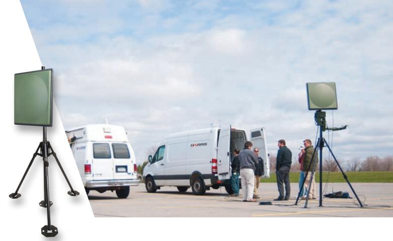
RAPIDLY DEPLOYABLE TWO-FOOT PANEL ANTENNA (4.4-5.875 GHZ)
