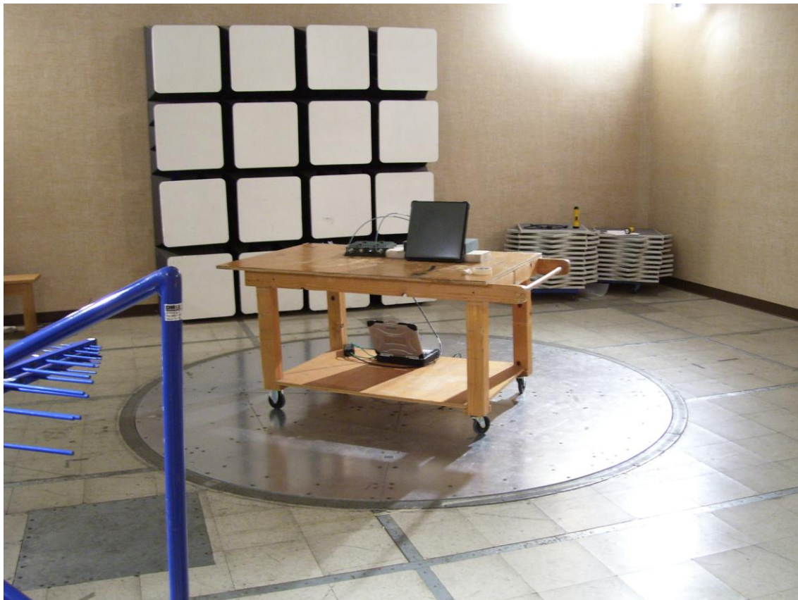
Figure 1: Prescan Radiated Emissions View w/ Remote External Antenna Connection
