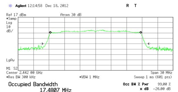
Transmit Freq Error 3.743 kHz x dB Bandwidth 19.204 MHz\*
