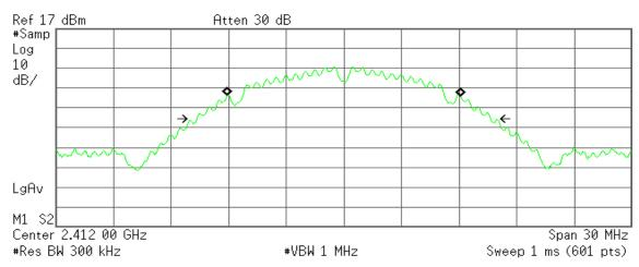
Occupied Bandwidth 12.1909 MHz Occ BW % Pwr 99.00 % x dB -26.00 dB
