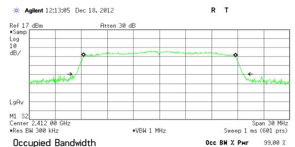
Transmit Freq Error -5.260 kHz x dB Bandwidth 19.244 MHz\*
