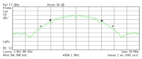
Occupied Bandwidth 12.2560 MHz Occ BW % Pwr 99.00 % **x dB** -26.00 dB
