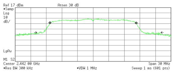
Occupied Bandwidth 16.5970 MHz Occ BW % Pwr 99.00 % x dB -26.00 dB
