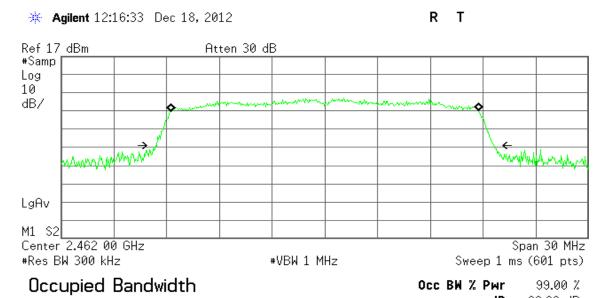
Transmit Freq Error 100.830 Hz x dB Bandwidth 19.220 MHz\*
