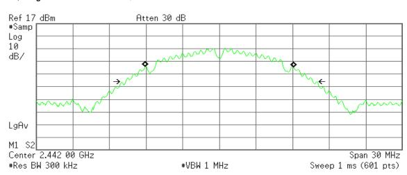
Occupied Bandwidth 12.2117 MHz Occ BW % Pwr 99.00 % x dB -26.00 dB
