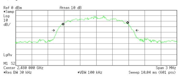
Occupied Bandwidth 1.1994 MHz Occ BW % Pwr 99.00 % x dB -26.00 dB
