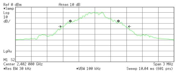
Occupied Bandwidth 905.5783 kHz Occ BW % Pwr 99.00 % **x dB** -26.00 dB
