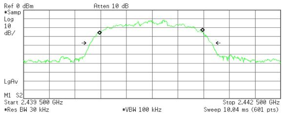
Occupied Bandwidth 1.1959 MHz Occ BW % Pwr 99.00 % x dB -26.00 dB
