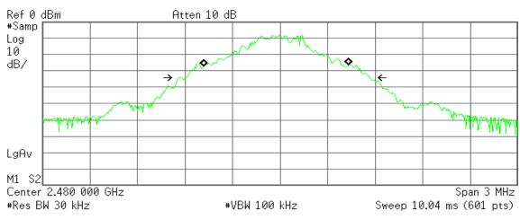
Occupied Bandwidth 910.1734 kHz Occ BW % Pwr 99.00 % x dB -26.00 dB
