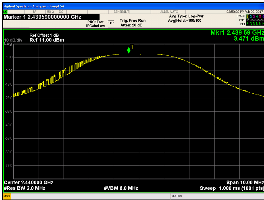
Figure 5 : Maximum peak conducted output power – IEEE 802.15.4 – 2440MHz
