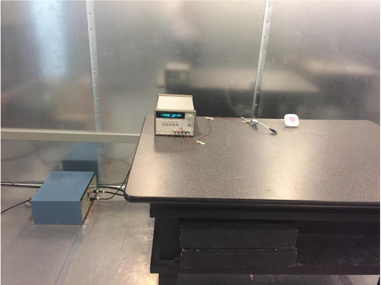
Figure 9: Conducted Emission Test Setup (Front)
