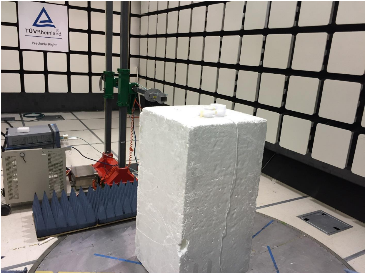
Figure 6: Test Setup for 18 GHz to 25GHz (Rear View)
