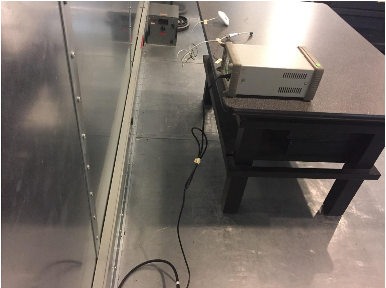
Figure 10: Conducted Emission Test Setup (Side)
