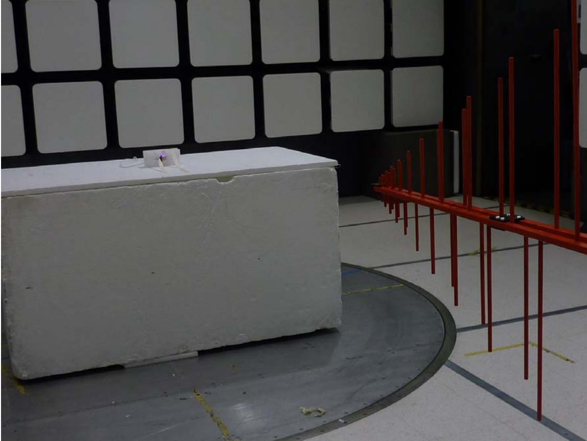
Figure 1: Test Setup for 30MHz to 1GHz (Front View)
