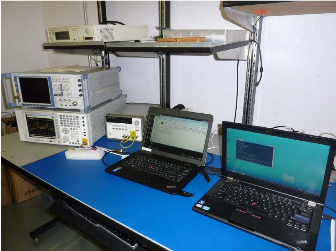
Figure 7: Conducted RF Test Setup
