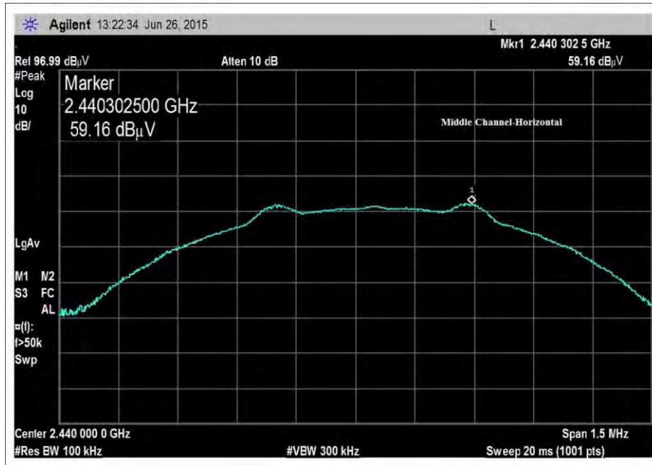
Middle Channel-Horizontal Polarization
