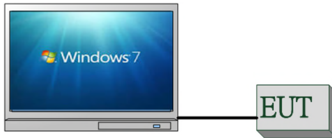
Fig. 2-1 Conducted (Antenna Port) & Radiated Emission & Conduction Configuration
