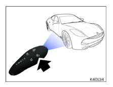
The vehicle security system, door locks, and ignition are controlled by the key fob. The doors and trunk can be either locked or unlocked using the key fob. The key fob is part of the immobilizer system. It operates in the manner described below.
