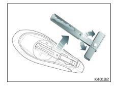
3. Remove the cover to expose the key blade nested in tray
