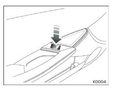
To open the door from the interior of the vehicle, press the switch on the interior door panel.
