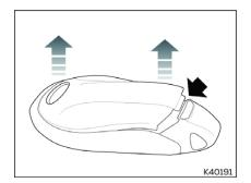
2. Carefully use tip of finger to release cover at opening
