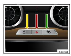
To lock or unlock all the doors while in the vehicle, press the master locking switch shown above.
