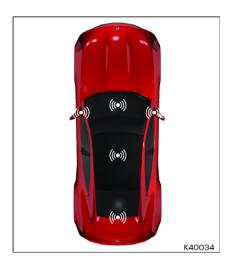
Antennas which detect the presence of the key fob are located in the following locations on your Revero:
