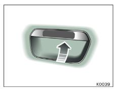
With the vehicle unlocked, lightly press the touch pad located behind the door handle to open the door.
