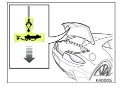
A T-shaped handle is located inside the trunk above the latch at the center of the trunk lid. This handle is made using a luminescent material that glows for hours after a brief exposure to ambient light.
