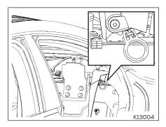
To manually open the trunk, remove the rear seat back on the driver side. A pull ring is located between the rear door and the rear head rest, just below the seatbelt retractor.
