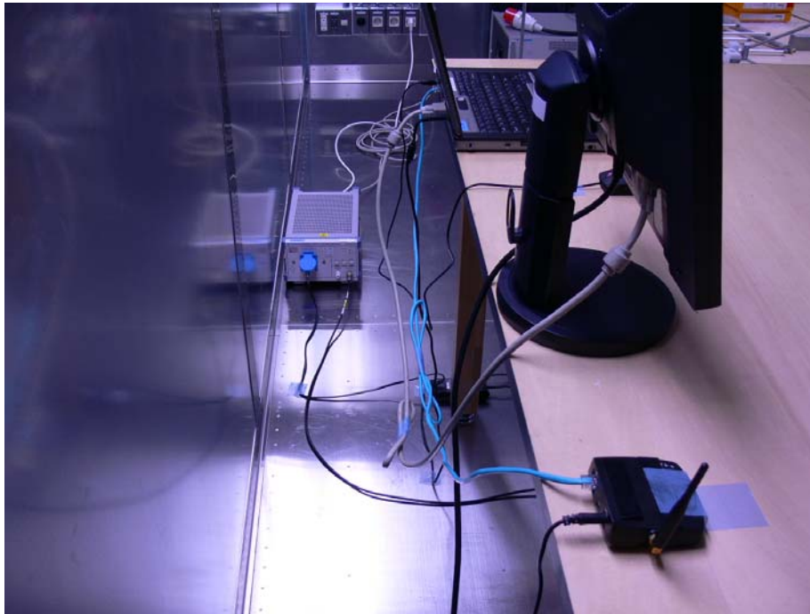
Photograph 8: Set-up for Conducted Emission, EUT Configuration
