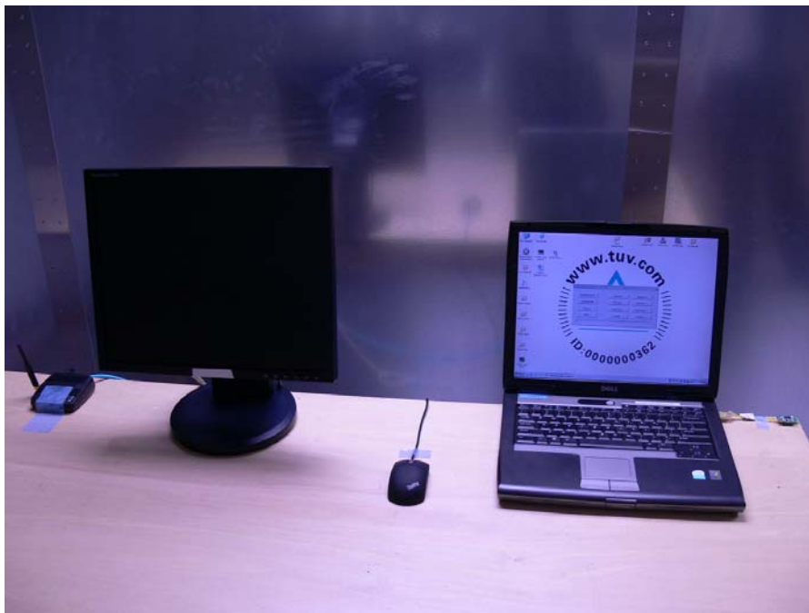
Photograph 7: Set-up for Conducted Emission, EUT Configuration
