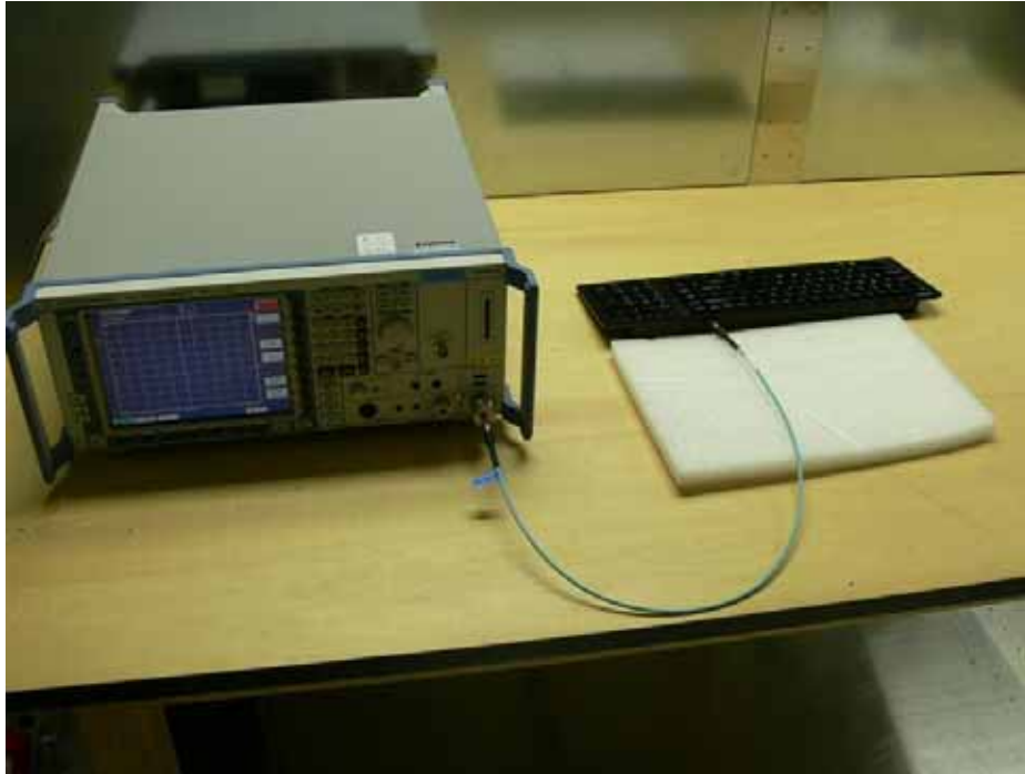
Photograph 1: Set-up for Conducted Emissions at Antenna Port
