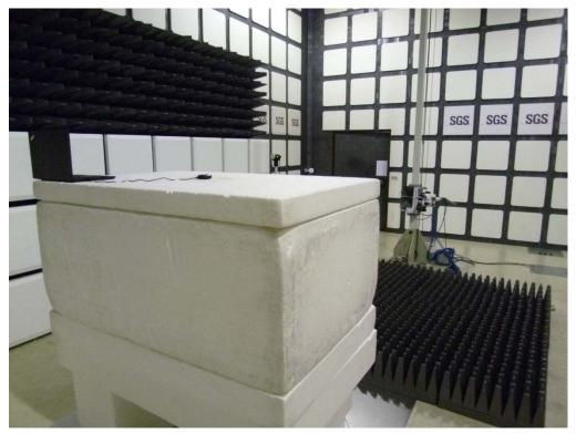
Radiated Emission Set up Photos (Front View)
