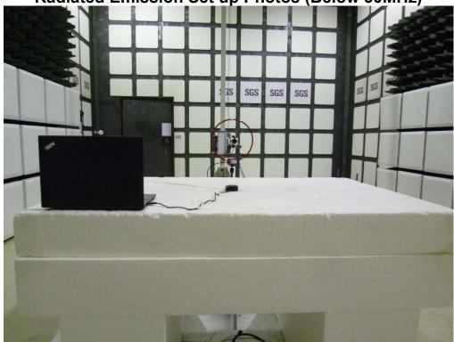
Radiated Emission Set up Photos (Below 1GHz)
