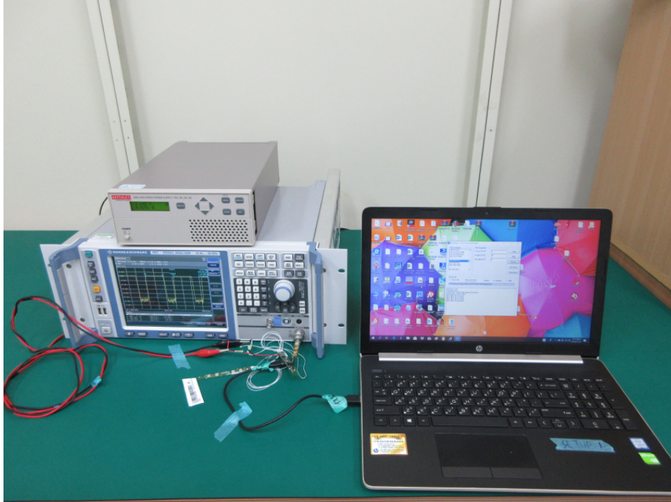
Photograph 7: Set-up for Conducted testing (View 1)
