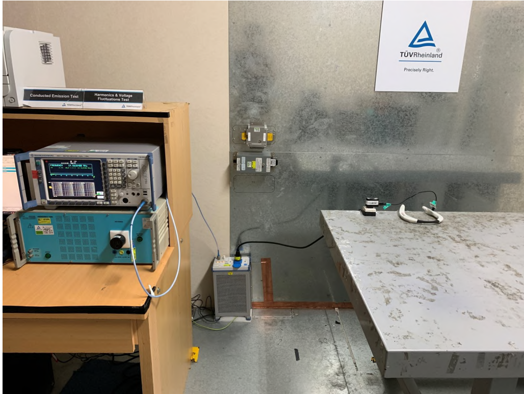
Photograph 10: Set-up for AC Mains Conducted testing (Back View)
