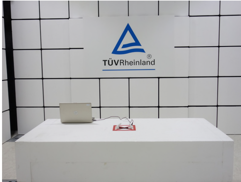
Photograph 1: Set-up for Spurious Emissions (Front View 1)
