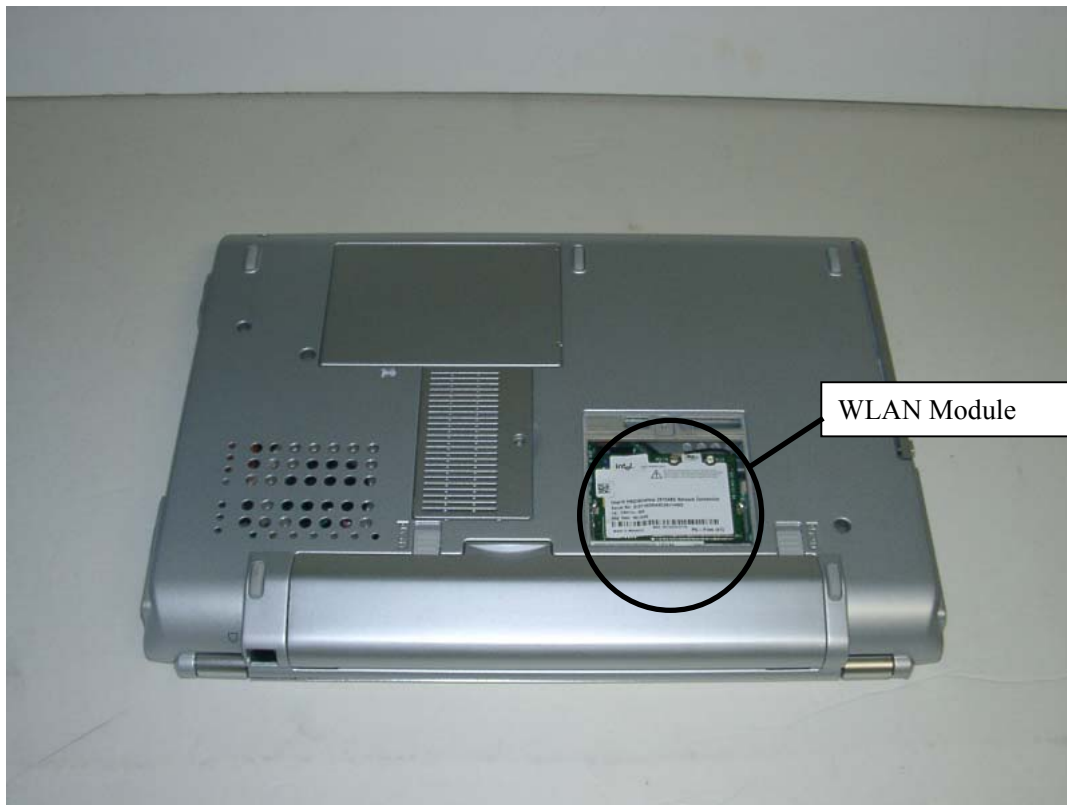
Location of WLAN module
