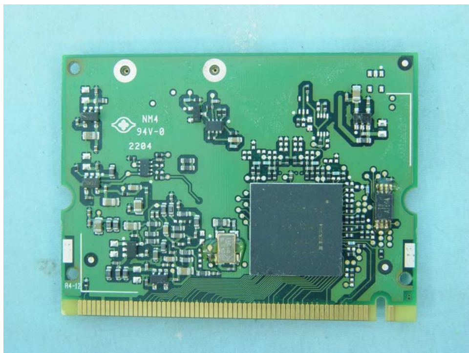
WLAN Module: Side B (without cover)
