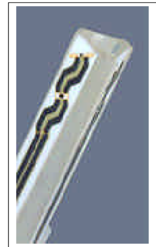
Inside view of ET3DV6 E-field Probe
