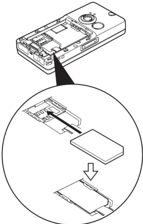
**4** Position the battery with the printed side up. Insert its top end as illustrated into slot ① and insert the other end into position ②.
