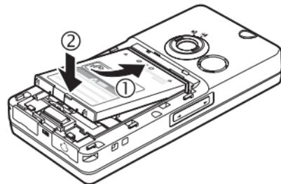
**5** Align the battery cover with the battery compartment as illustrated and slide it in the direction of the arrow until it clicks.
