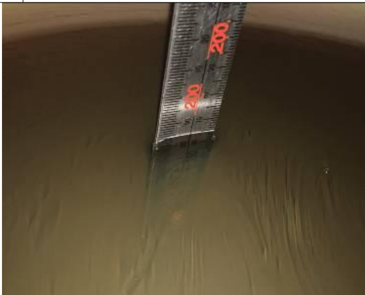
Liquid depth for SAR Measurement
