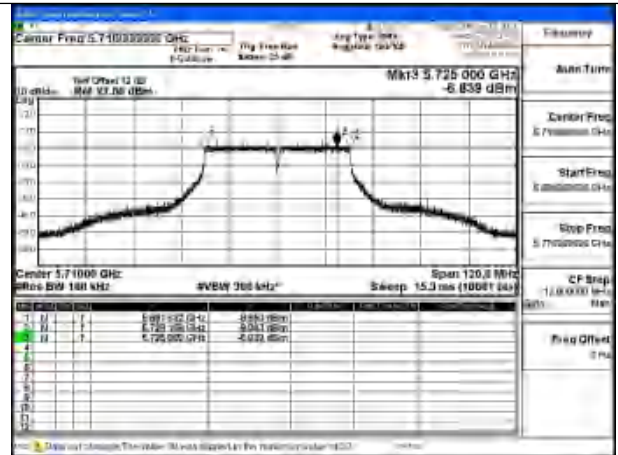
Mode:802.11ac VHT40 Frequency:5710MHz Ant:Chain1 scope:NII2C
