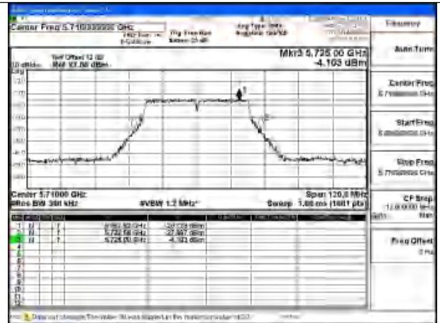
Mode:802.11n HT40 Frequency:5710MHz Ant:Chain1 scope:NII2C
