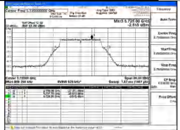
Mode:802.11n HT20 Frequency:5720MHz Ant:Chain1 scope:NII2C
