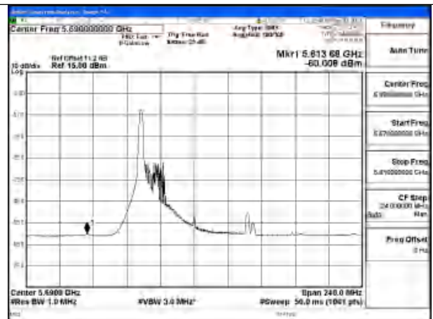
Mode:802.11be EHT80 Tone:26TL Frequency:5690MHz Ant:Chain1 scope:NII2C
