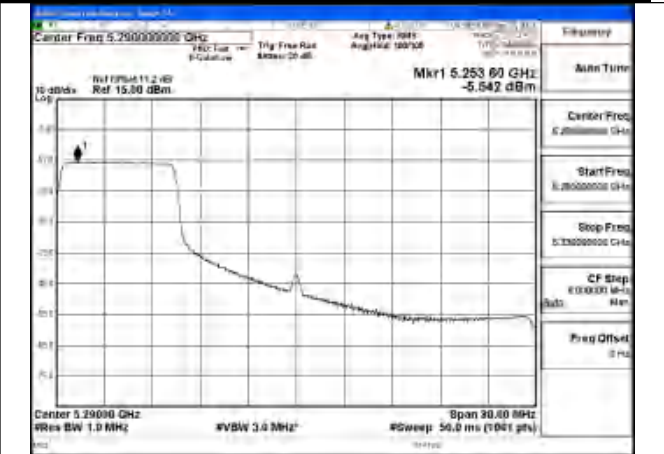
Mode:802.11be EHT80 Tone:242T Frequency:5290MHz Ant:Chain1
