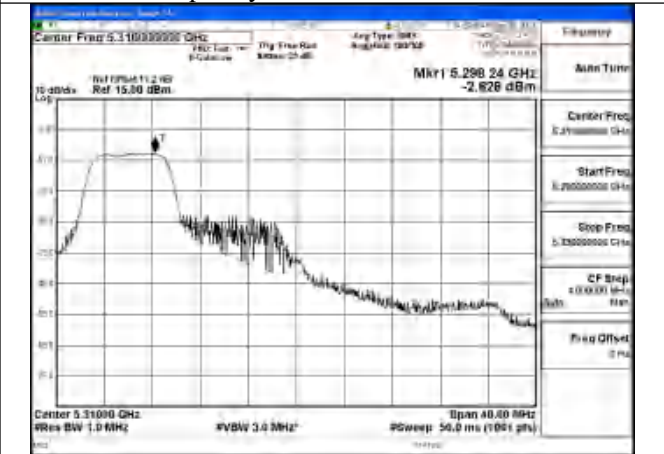
Mode:802.11be EHT40 Tone:26+52 Frequency:5310MHz Ant:Chain1
