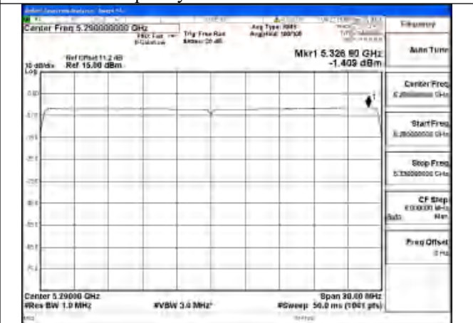
Mode:802.11be EHT80 Tone:996T Frequency:5290MHz Ant:Chain1
