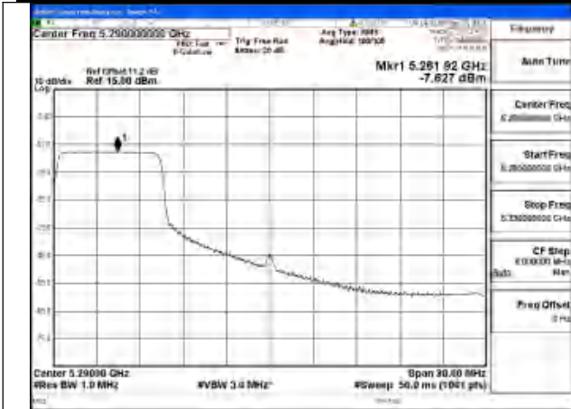
Mode:802.11be EHT80 Tone:242T Frequency:5290MHz Ant:Chain0
