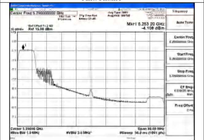
Mode:802.11be EHT80 Tone:106T Frequency:5290MHz Ant:Chain1
