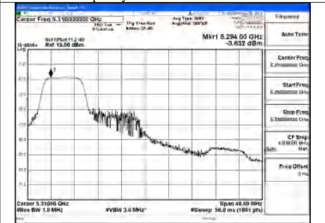
Mode:802.11be EHT40 Tone:26+52 Frequency:5310MHz Ant:Chain0
