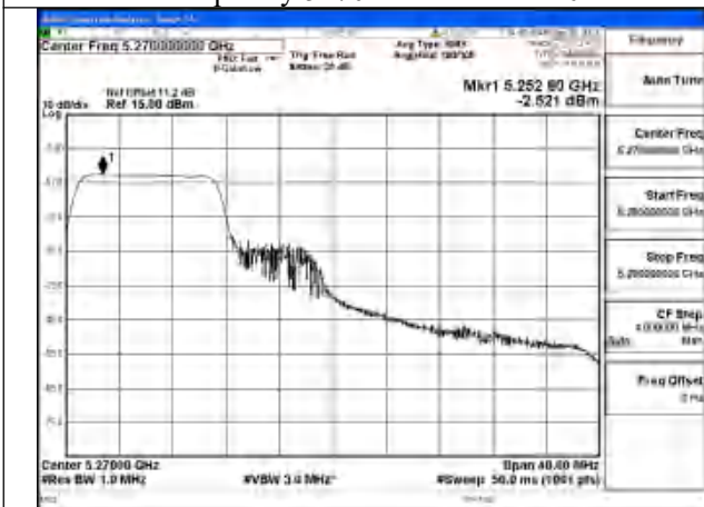
Mode:802.11be EHT40 Tone:26+106 Frequency:5270MHz Ant:Chain1
