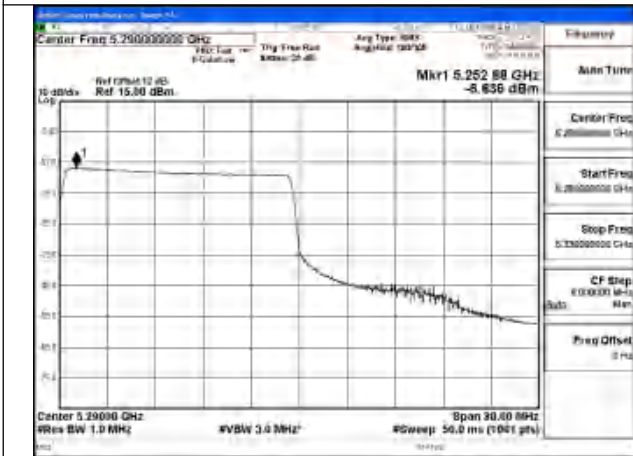
Mode:802.11ax HE80 Tone:484T Frequency:5290MHz Ant:Chain1
