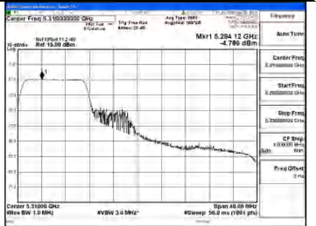
Mode:802.11be EHT40 Tone:26+106 Frequency:5310MHz Ant:Chain0
