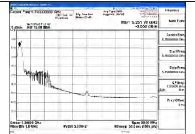
Mode:802.11be EHT80 Tone:26T Frequency:5290MHz Ant:Chain1
