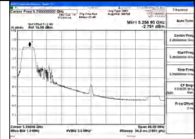
Mode:802.11be EHT80 Tone:26+52 Frequency:5290MHz Ant:Chain1
