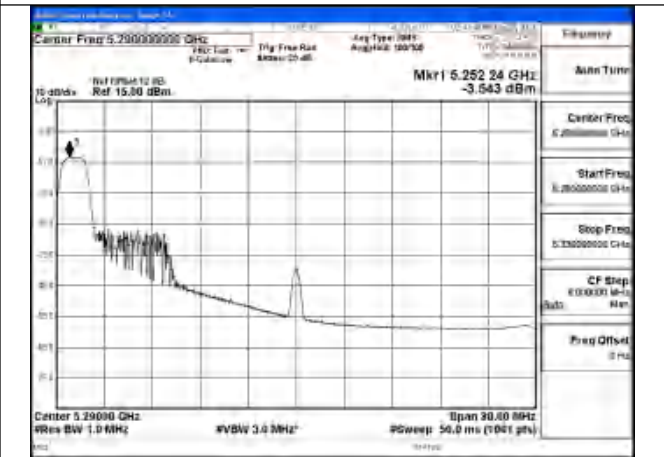
Mode:802.11ax HE80 Tone:52T Frequency:5290MHz Ant:Chain0
