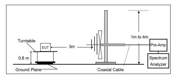
Radiated Emission Test Set-Up, Frequency Above 1GHz.
