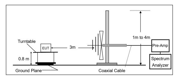
Radiated Emission Test Set-Up, Frequency Above 1GHz.
