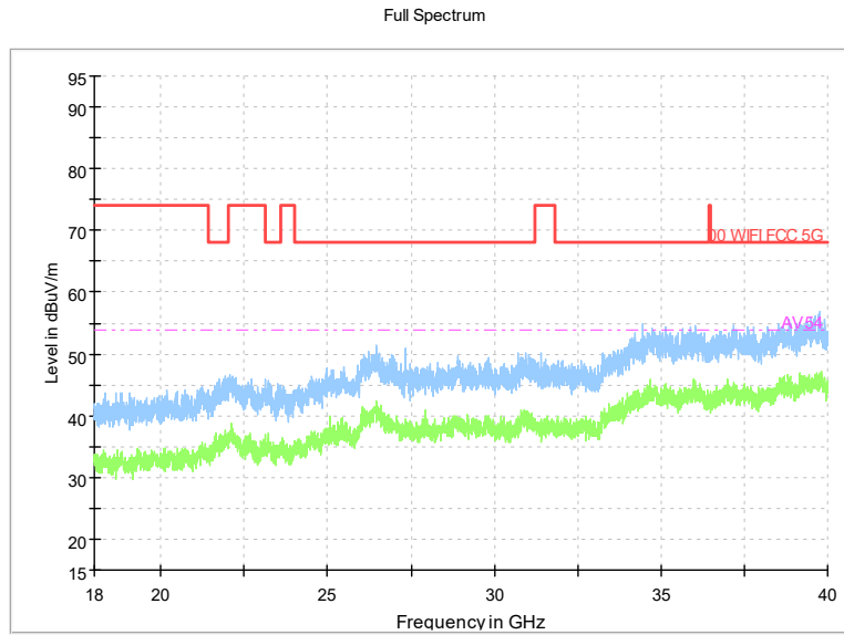
Frequency Range: 18GHz -40GHz Detector: Av mode and PK mode Modulation type: 802.11a
