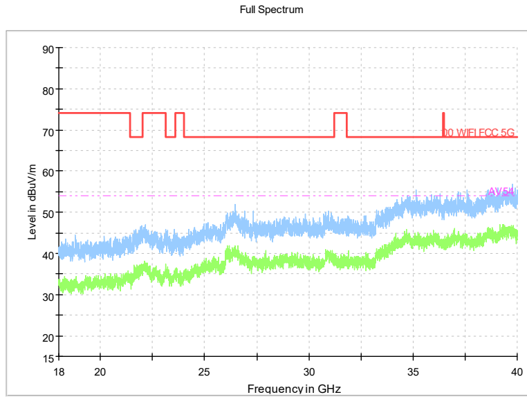
Frequency Range: 18GHz -40GHz Detector: Av mode and PK mode Test Mode: 802.11ac(VHT20)
