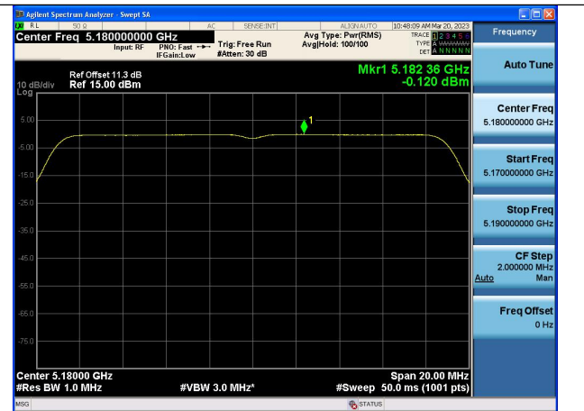
Mode:802.11ac VHT20 Frequency:5180MHz Ant:Chain1
