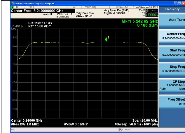
Mode:802.11a Frequency:5240MHz Ant:Chain0
