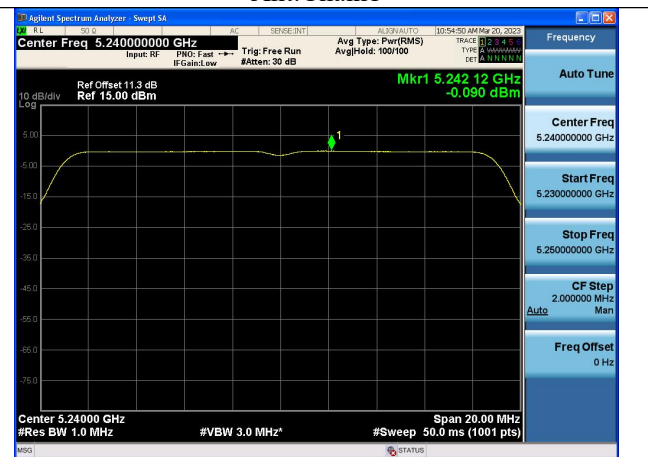
Mode:802.11ac VHT20 Frequency:5240MHz Ant:Chain1
