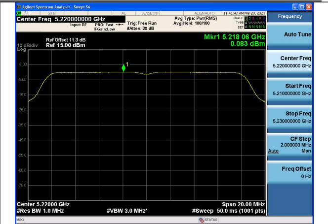
Mode:802.11a Frequency:5220MHz Ant:Chain0
