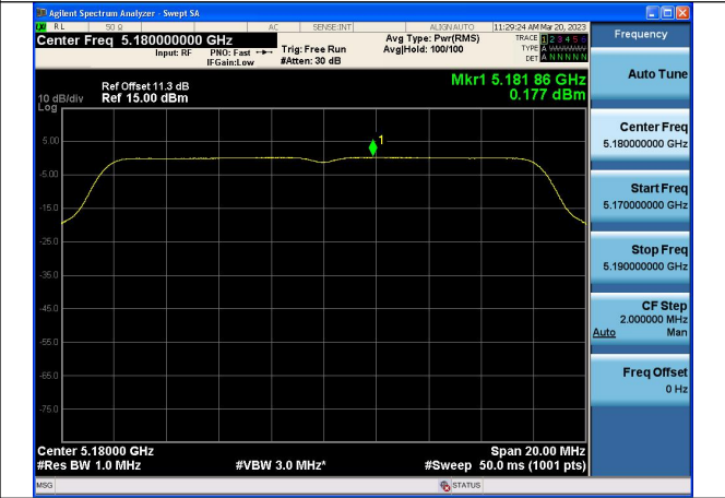
Mode:802.11a Frequency:5180MHz Ant:Chain1
