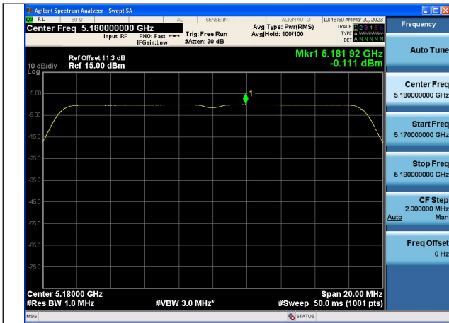
Mode:802.11ac VHT20 Frequency:5180MHz Ant:Chain0
