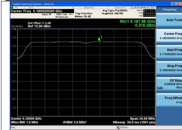
Mode:802.11a Frequency:5180MHz Ant:Chain0
