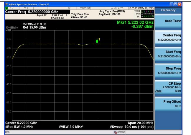
Mode:802.11ac VHT20 Frequency:5220MHz Ant:Chain0
