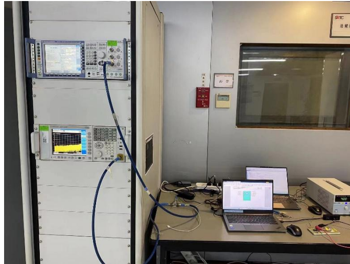
RF Conducted Test setup (GSM/WCDMA)
