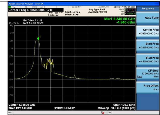
Mode:802.11ax HE80 Tone:52T Frequency:6385MHz Chain1
