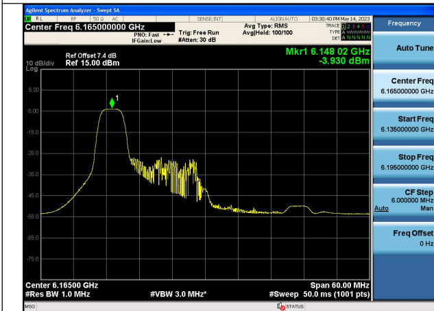
Mode:802.11ax HE40 Tone:52T Frequency:6165MHz Chain1
