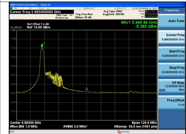
Mode:802.11ax HE80 Tone:26T Frequency:5985MHz Chain1
