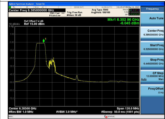
Mode:802.11ax HE80 Tone:106T Frequency:6385MHz Chain1
