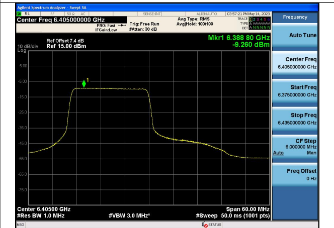
Mode:802.11ax HE40 Tone:242T Frequency:6405MHz Chain1
