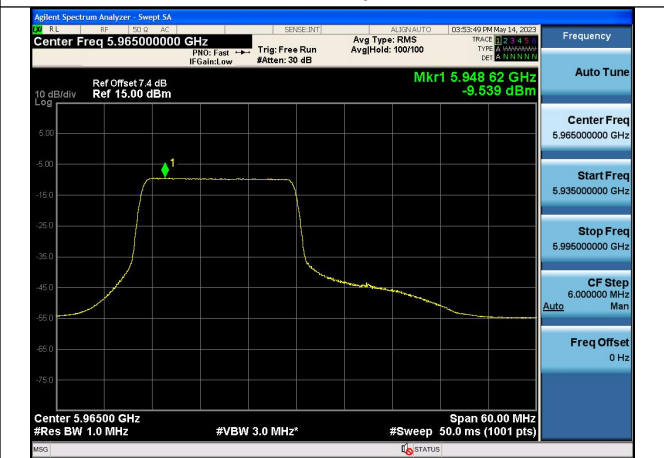
Mode:802.11ax HE40 Tone:242T Frequency:5965MHz Chain1
