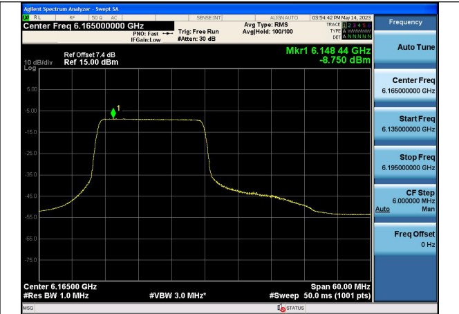
Mode:802.11ax HE40 Tone:242T Frequency:6165MHz Chain0
