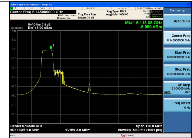
Mode:802.11ax HE80 Tone:106T Frequency:6145MHz Chain0
