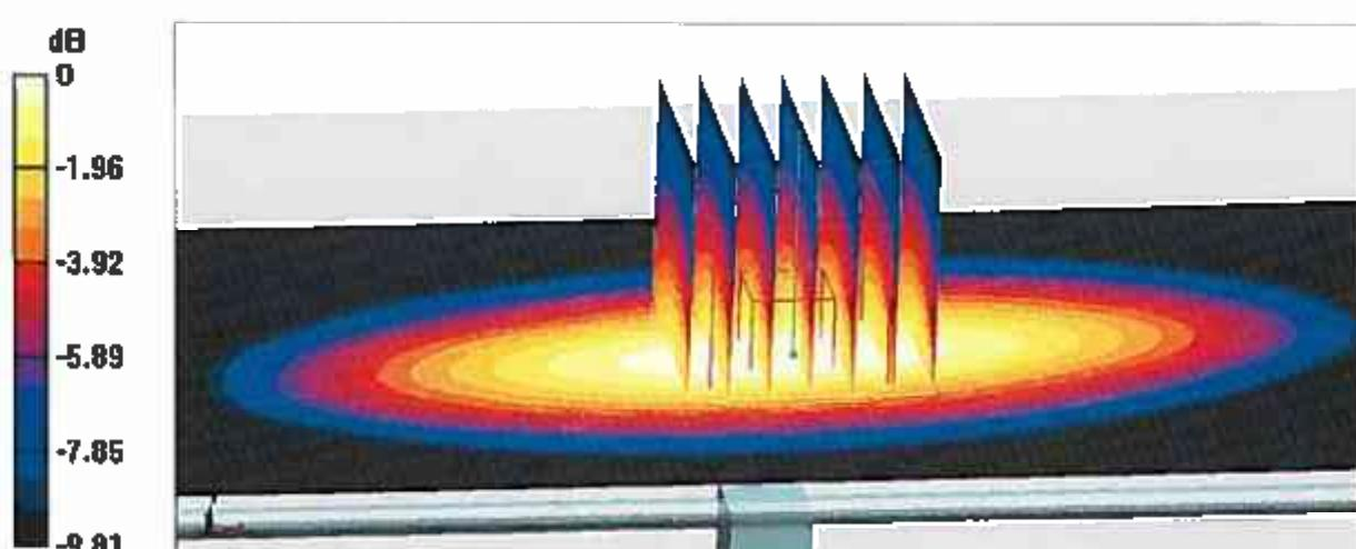
$$0 \text{ dB} = 3.08 \text{ W/kg} = 4.89 \text{ dBW/kg}$$
