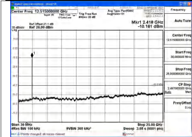
Mode:802.11n HT20 Frequency:2412MHz Ant:Chain0
