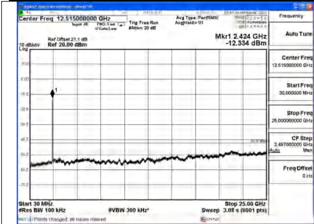
Mode:802.11n HT40 Frequency:2422MHz Ant:Chain0
