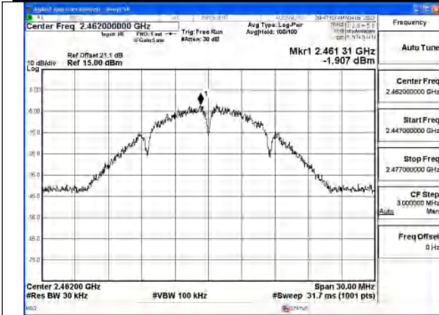
Mode:802.11b Frequency:2462MHz Ant:Chain0
