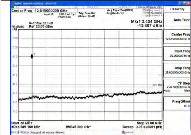
Mode:802.11n HT40 Frequency:2437MHz Ant:Chain1
