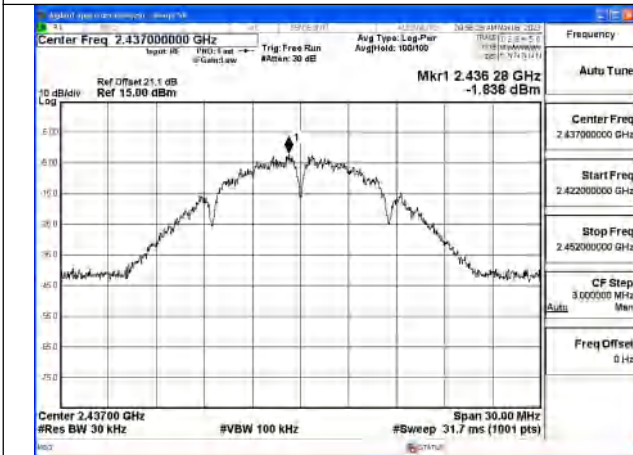
Mode:802.11b Frequency:2437MHz Ant:Chain1
