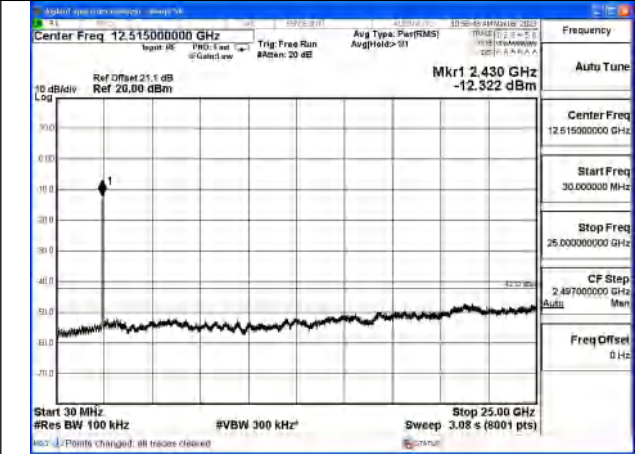
Mode:802.11n HT40 Frequency:2422MHz Ant:Chain1
