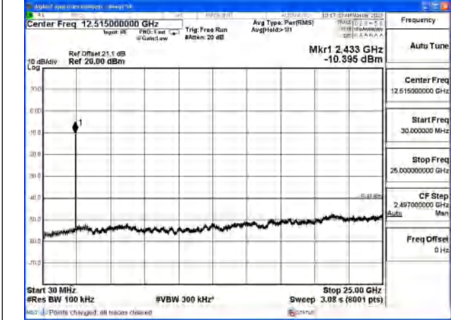
Mode:802.11n HT20 Frequency:2437MHz Ant:Chain1
