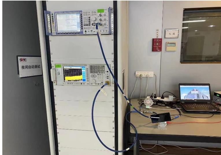
RF Conducted Test setup (GSM/WCDMA/LTE)
