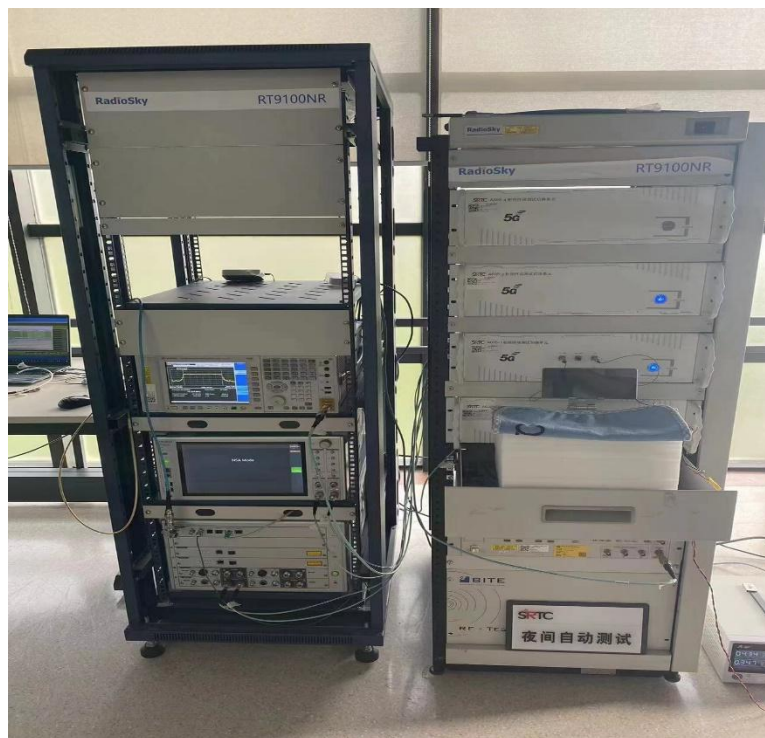
RF Conducted Test setup (NR)
