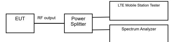
Test procedure: KDB 971168 D01 v03r01 – Section 6.0
