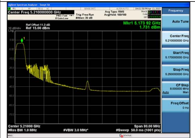
Mode:802.11ax HE80 Tone:52T Frequency:5210MHz Ant:Chain1
