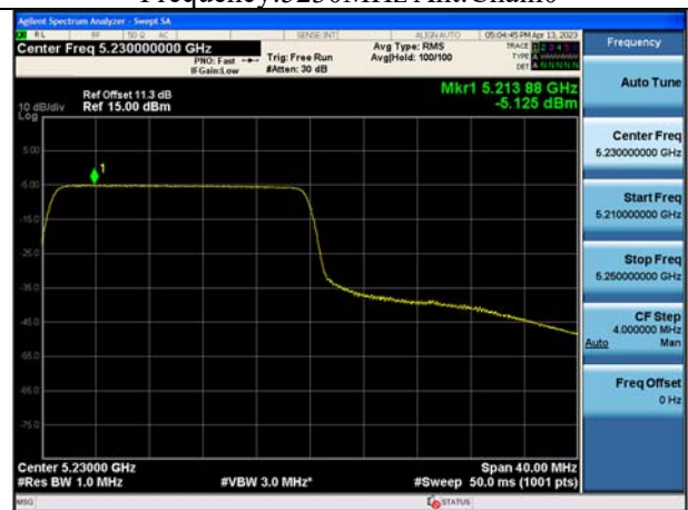
Mode:802.11ax HE40 Tone:242T Frequency:5230MHz Ant:Chain1
