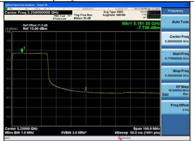
Mode:802.11ax HE160 Tone:484T Frequency:5250MHz Ant:Chain1
