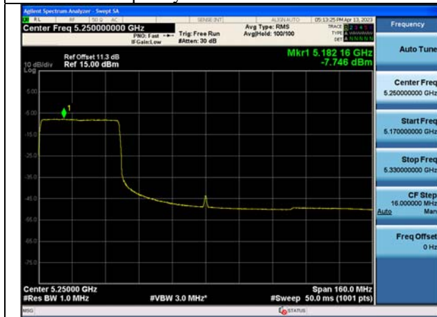
Mode:802.11ax HE160 Tone:484T Frequency:5250MHz Ant:Chain0
