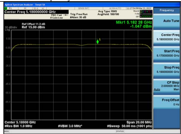
Mode:802.11ax HE20 Tone:242T Frequency:5180MHz Ant:Chain1
