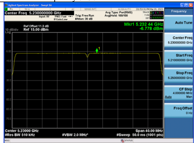
Mode:802.11ax HE40 Tone:484T Frequency:5230MHz Ant:Chain0
