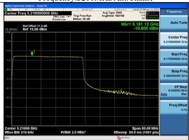
Mode:802.11ax HE80 Tone:484T Frequency:5210MHz Ant:Chain1
