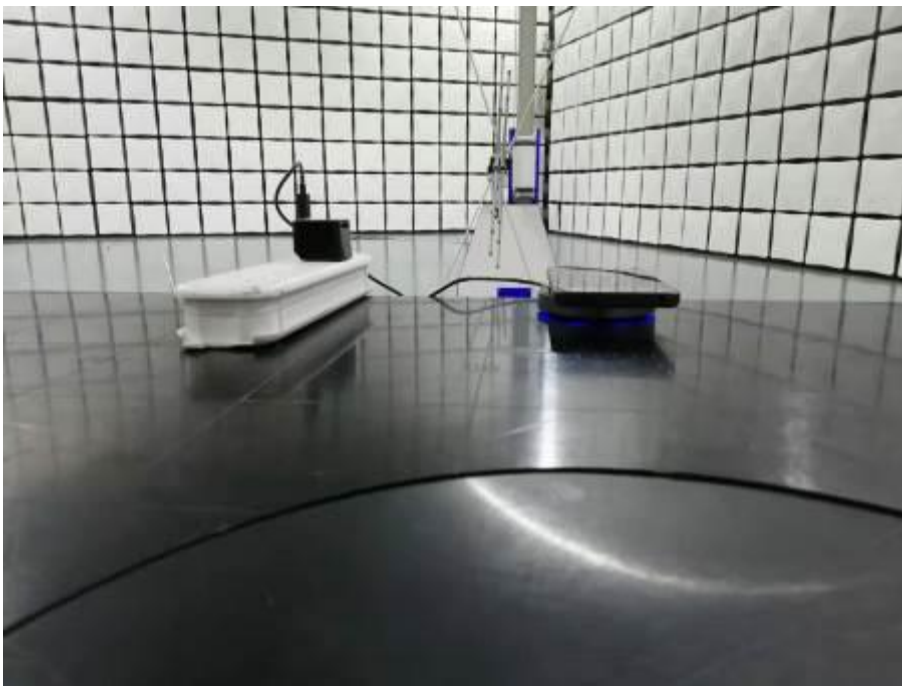
Radiated Emissions Test Setup (30-1000MHz)
