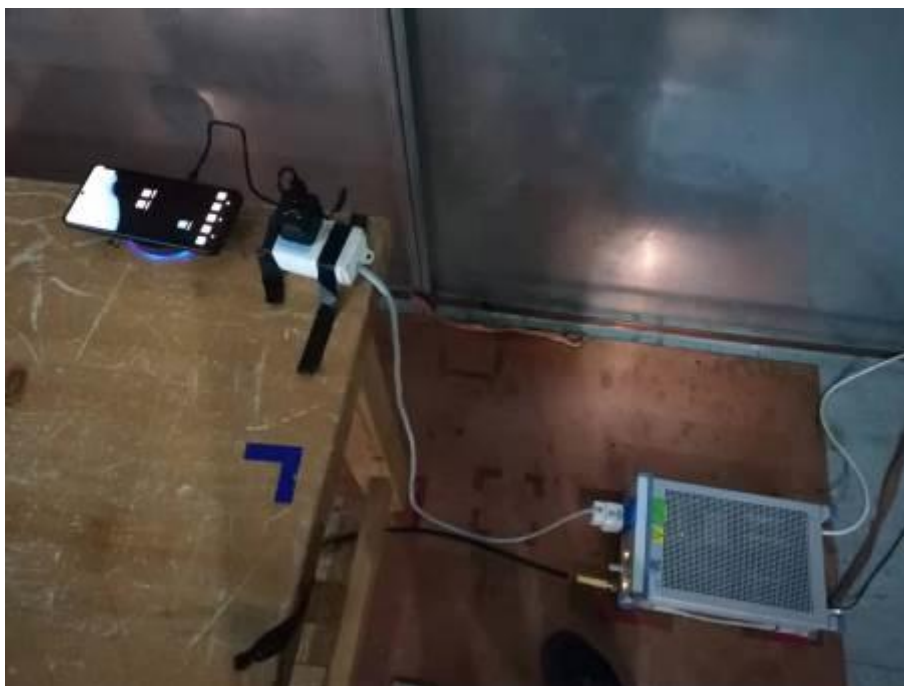
Conducted Emissions Test Setup
