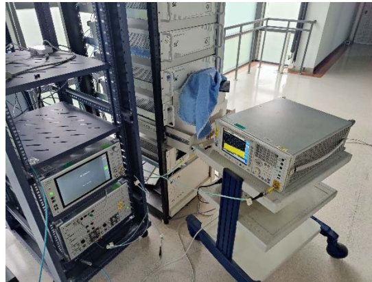
RF Conducted Test setup (NR)
