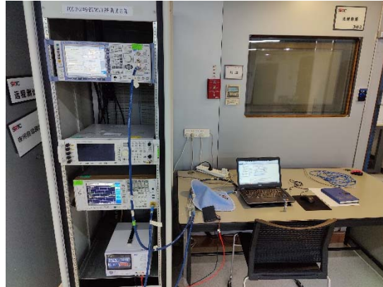
RF Conducted Test setup (GSM/WCDMA/LTE)
