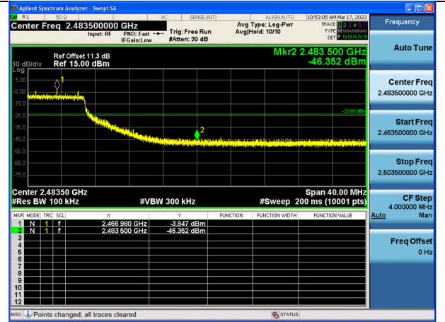
Test Mode:802.11n HT40 2452MHz Chain1
