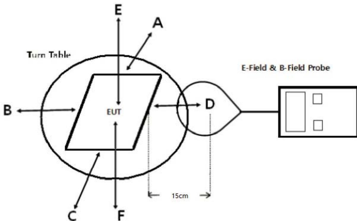
Note: position F of the charging device shall be test with underside up.
