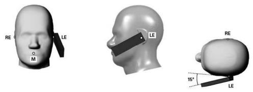
Fig-4.3 Illustration for Tilted Position
