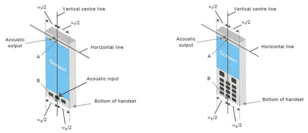
Illustration for Handset Vertical and Horizontal Reference Lines Fig-4.1
