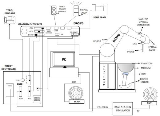
Fig-3.1 SPEAG DASY6 System Setup
