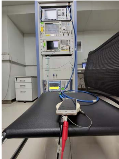
RF Conducted Test setup (GSM/WCDMA/LTE)
