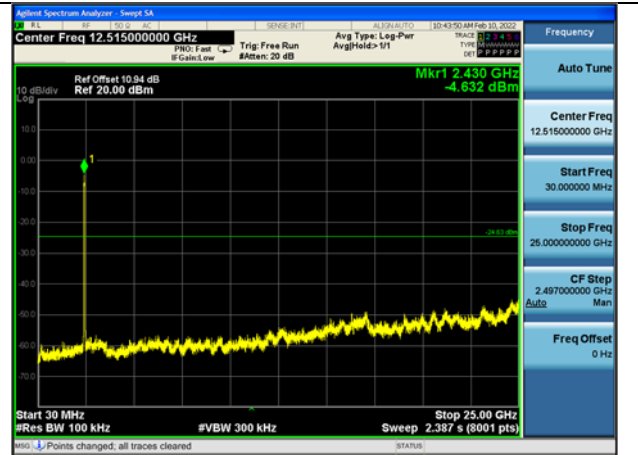
Test Mode:802.11n HT40 2437MHz Chain0
