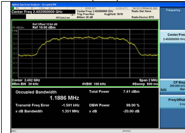
Test Mode: \pi/4 DQPSK(2DH5) 2402 MHz
