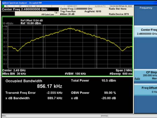
Test Mode:GFSK(DH5) 2480 MHz
