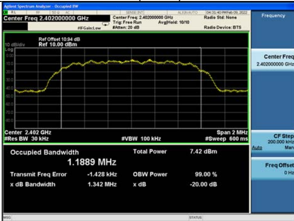
Test Mode: \pi/4 DQPSK(2DH5) 2402 MHz
