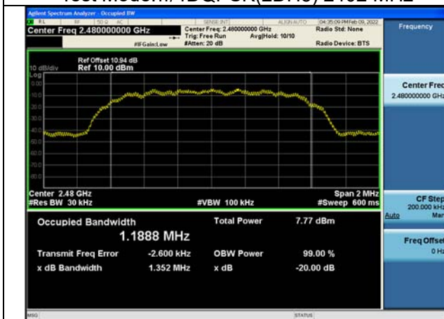
Test Mode: \pi/4 DQPSK(2DH5) 2480 MHz
