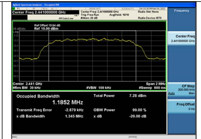
Test Mode: \pi/4 DQPSK(2DH5) 2441 MHz
