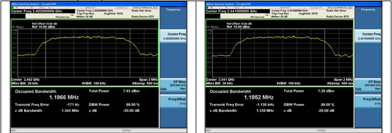
Test Mode:8DPSK(3DH5) 2402 MHz
