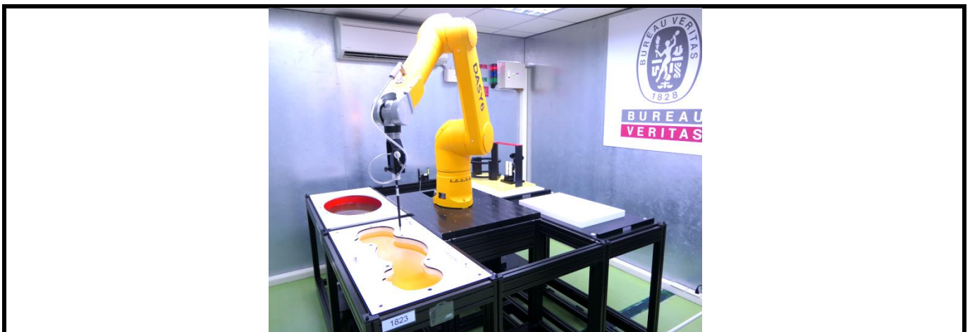
Fig-3.2 SPEAG DASY6 System
