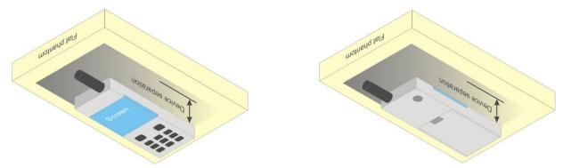
Fig-4.4 Illustration for Body Worn Position
