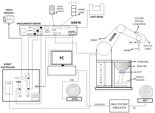
Fig-3.1 SPEAG DASY6 System Setup
