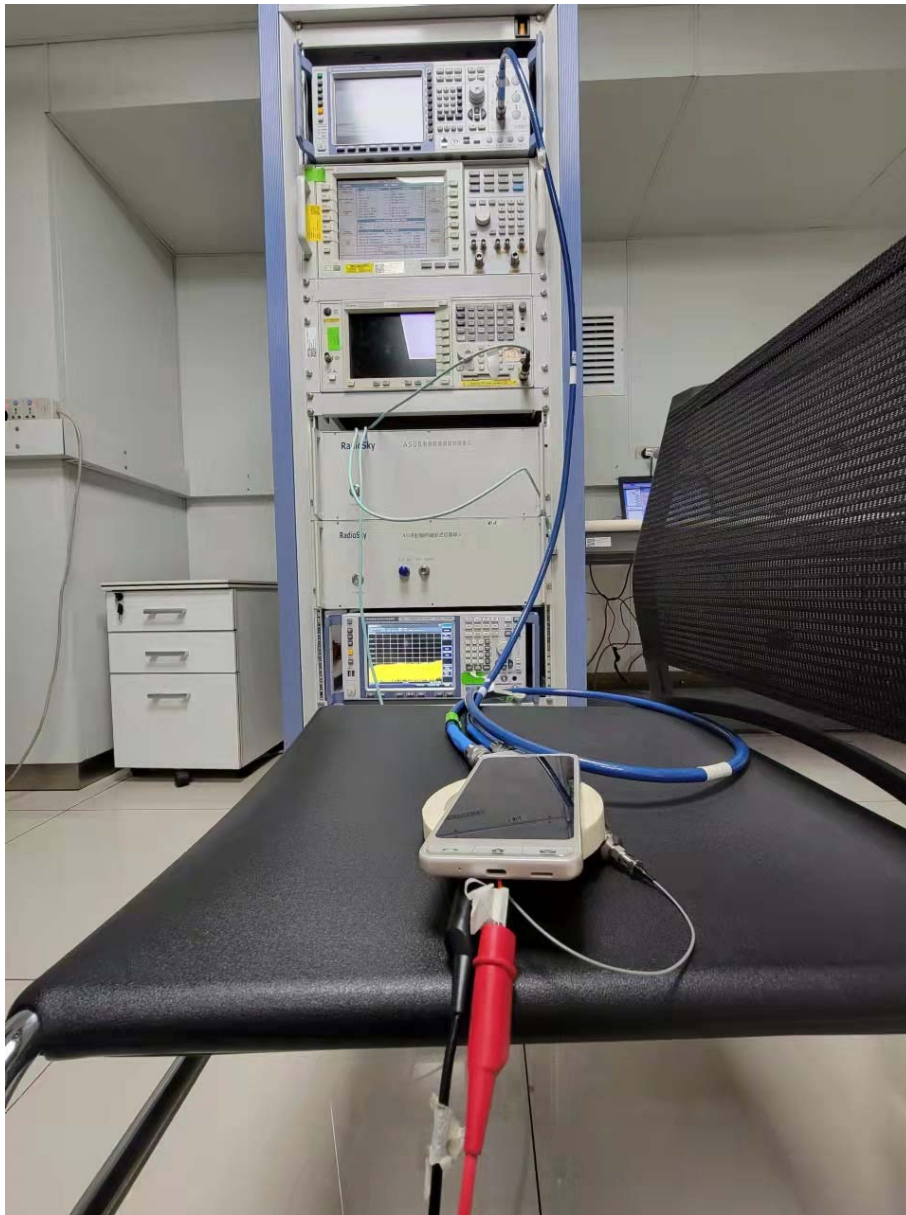
RF Conducted Test setup (GSM/WCDMA/LTE)
