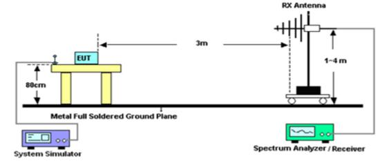
For radiated test above 1GHz
